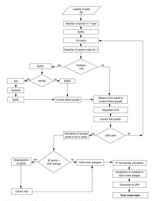
Figure 2. Crown delineation process using the POSTGRES function.
