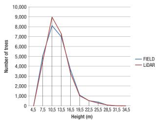
Figure 5. Height distribution for field trees & LiDAR delineated trees. where:
