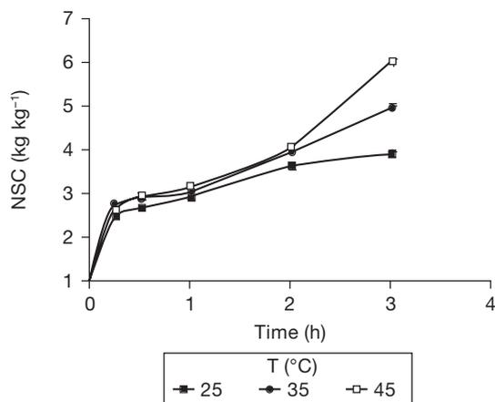
**Figure 5.** Normalized solid content (*NSC*) evolution with time at different temperatures. OD: 26% w/w salt concentration and diameter of samples of 7 mm.
