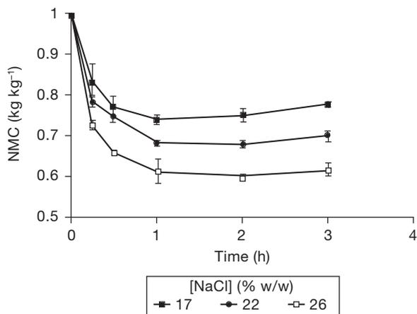
**Figure 3.** Normalized moisture content (*NMC*) evolution with time at different NaCl concentrations. OD: 25°C and diameter of samples 7 mm.
