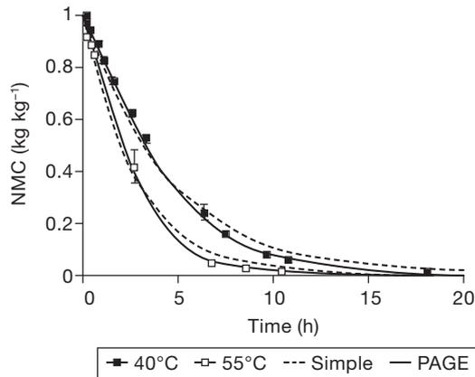
**Figure 6.** Influence of temperature on the convective drying of samples with diameter of 7 mm.
