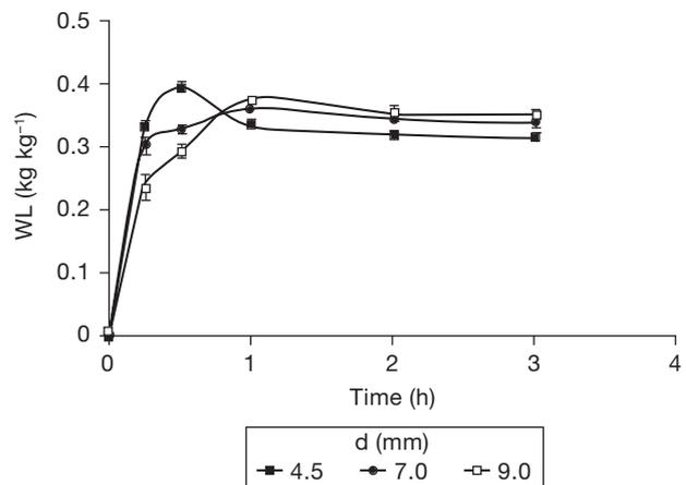
**Figure 1.** Water loss ( $WL$ ) evolution with time for samples of different diameters ( $d$ ). OD: 26% w/w NaCl concentration and 45°C.
