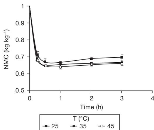
**Figure 2.** Normalized moisture content (*NMC*) evolution with time at different temperatures. OD: 26% w/w salt concentration and diameter of samples of 7 mm.
