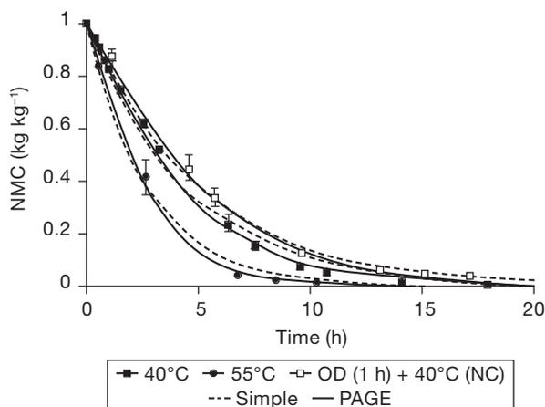
**Figure 8.** Normalized moisture content (*NMC*) evolution with time in convective drying (NC: 40 and 55°C, diameter of sample 7 mm) and in the combined process of osmotic dehydration (OD: 1 h, 26% w/w salt concentration, diameter of samples of 7 mm and 25°C) and convective drying (NC: 40°C and diameter of samples of 7 mm).
