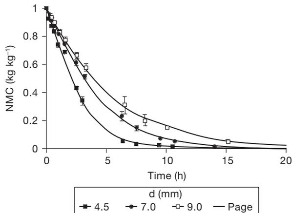
**Figure 7.** Influence of the diameter of samples on convective drying at 40°C.
