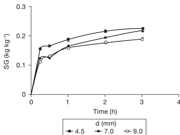
**Figure 4.** Solid gain (*SG*) evolution with time for different sample diameters (*d*). OD: 26% w/w salt concentration and 45°C.
