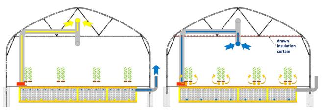
Figure 1. Charging the heat accumulator during a warm day (left) and discharging the accumulator for plant heating during the night or cold day (right).
