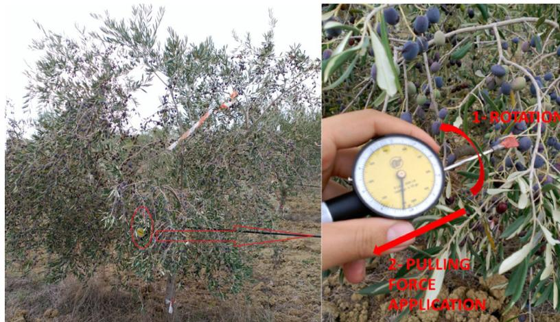
**Figure 1.** Dynamometer with modified hook for make stalk twisting before fruit detachment force (FDF) measurement
