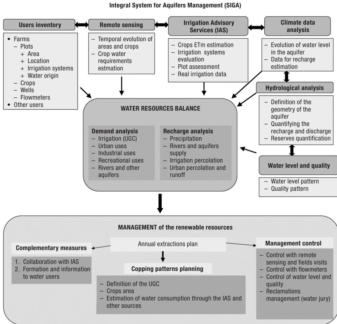
**Figure 2.** Flow chart of the integrated aquifer management system. UGC: Common Management Units.
