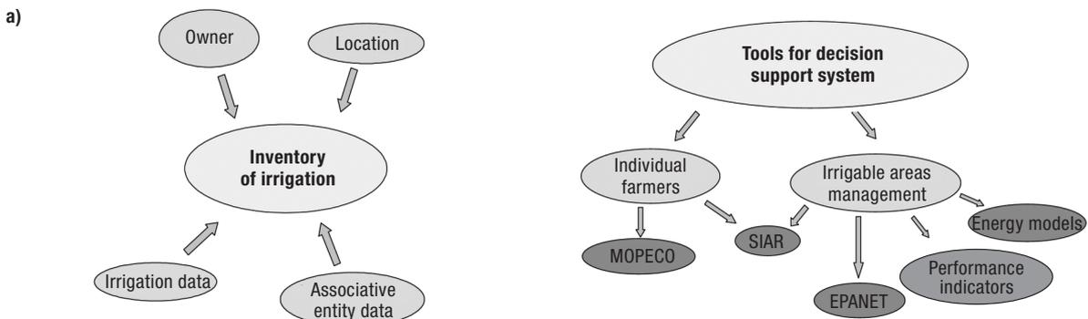
**Figure 3.** Diagram of a) irrigation inventory data and b) modules for calculating management improvement. MOPECO (Modelo de OPTimización ECONómica; Ortega *et al.*, 2004a). SIAR (Servicio Integral de Asesoramiento al Regante). EPANET (Risk Reduction Engineering Laboratory, Office of Research and Development, U.S. Environmental Protection Agency, Cincinnati, Ohio).
