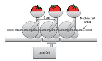
Figure 3. Scheme of dynamic weighing subsystem.
