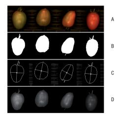
**Figure 5.** Image processing on industrial PC. A) colour image, B) threshold, C) edge, centre and diameter detection, D) green channel masked.
