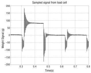
Figure 4. Typical weighing cycle.
