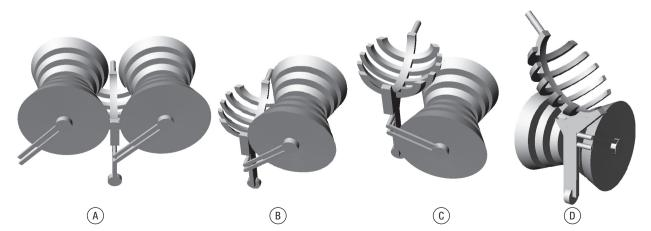
**Figure 2.** Detailed three-dimensional bucket. Positions: A) two adjacent buckets fitting (rotation position for image sampling), B) view of a bucket (rotation position for image sampling), C) weighing, D) tilt (expulsion of fruit).
