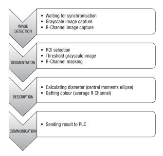
Figure 6. Duty cycle of image processing PC.
