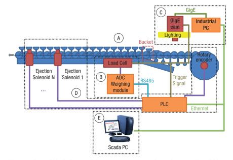
**Figure 1.** General block diagram. Subsystems: A) transportation and support, B) weighing, C) vision, D) control of synchronisation and ejection, E) monitoring.
