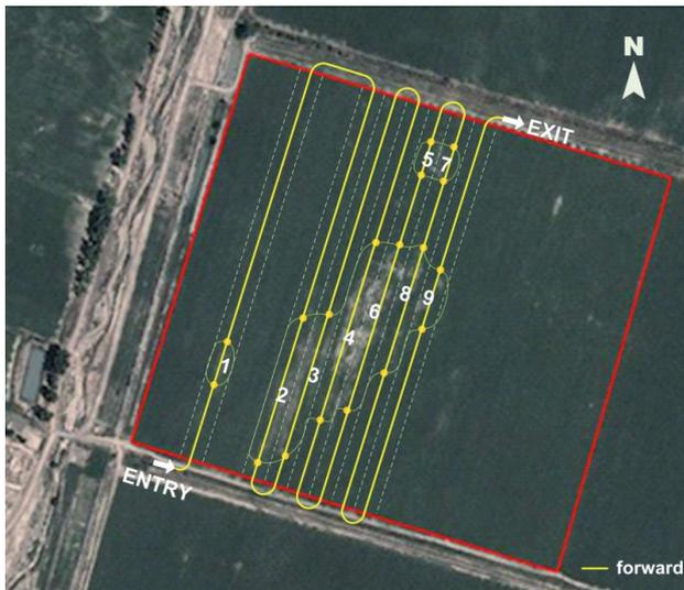
**Figure 6.** Robot paths for covering nine patches with Bochtis's method.
