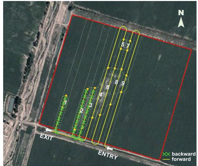
Figure 5. Optimal robot paths for covering nine patches.
