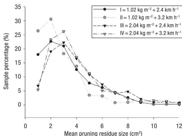
**Figure 6.** Distribution of the mean values for size of pruning residues for different quantities of pruning residues ( $\text{kg m}^{-2}$ ) and chopping speeds ( $\text{km h}^{-1}$ ) determined by image analysis.
