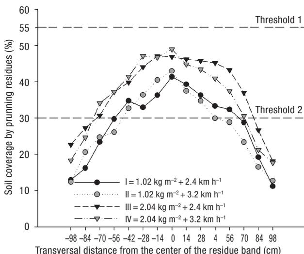
**Figure 4.** Transverse distribution of the mean values of the soil cover percentage as a function of the distance from the center of the chopping band for different pruning residue quantities ( $\text{kg m}^{-2}$ ) and chopping speeds ( $\text{km h}^{-1}$ ) as determined by image analysis.
