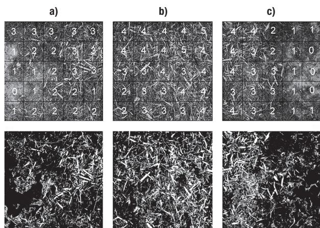
**Figure 2.** Examples of images taken under shielded conditions. Processing using the visual estimation method (top row) and digital image analyses (bottom row). a), b), and c) correspond to the left, central, and right surfaces of the sample area, respectively.
