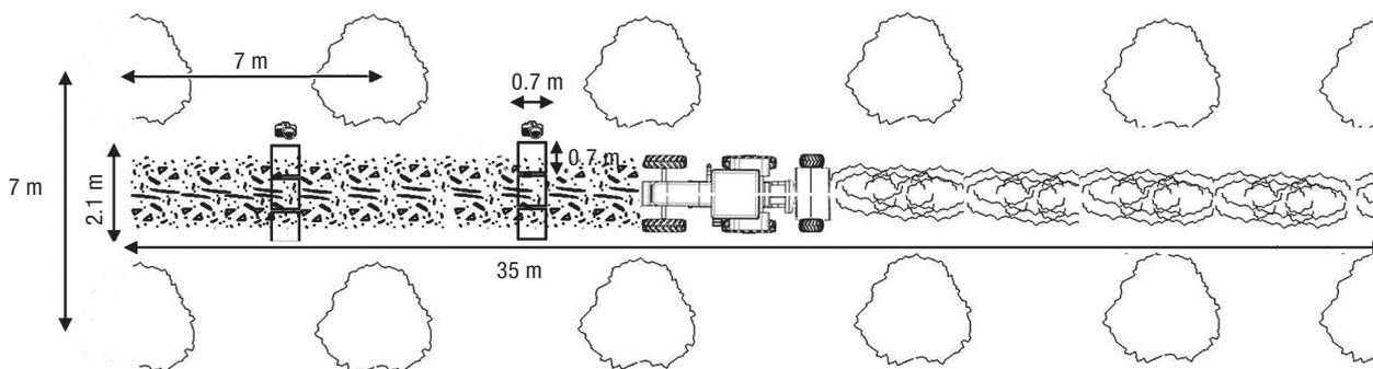
**Figure 1.** Block configuration for field image acquisition of the chopped pruning residues in an olive orchard.
