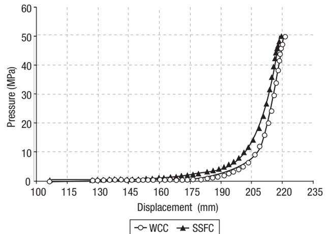
**Figure 6.** Force-displacement plot comparison between SSFC and WCC obtained applying 50 MPa for 40 s.
