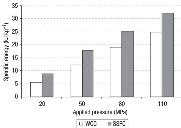
**Figure 5.** Average specific compression energy values (kJ kg<sup>-1</sup>) required for densification of WCC and SSFC obtained using different pressure levels (20, 50, 80 and 110 MPa).
