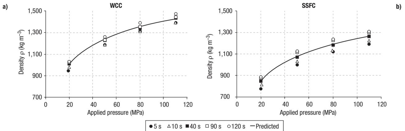
**Figure 2.** Effect of pressure and pressure application time on the density of WCC (a) and SSFC (b).
