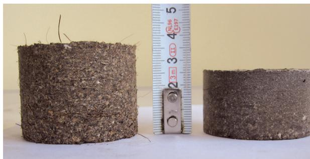
**Figure 1.** Samples obtained applying 50 MPa for 40 s (SSFC on the left and WCC on the right).
