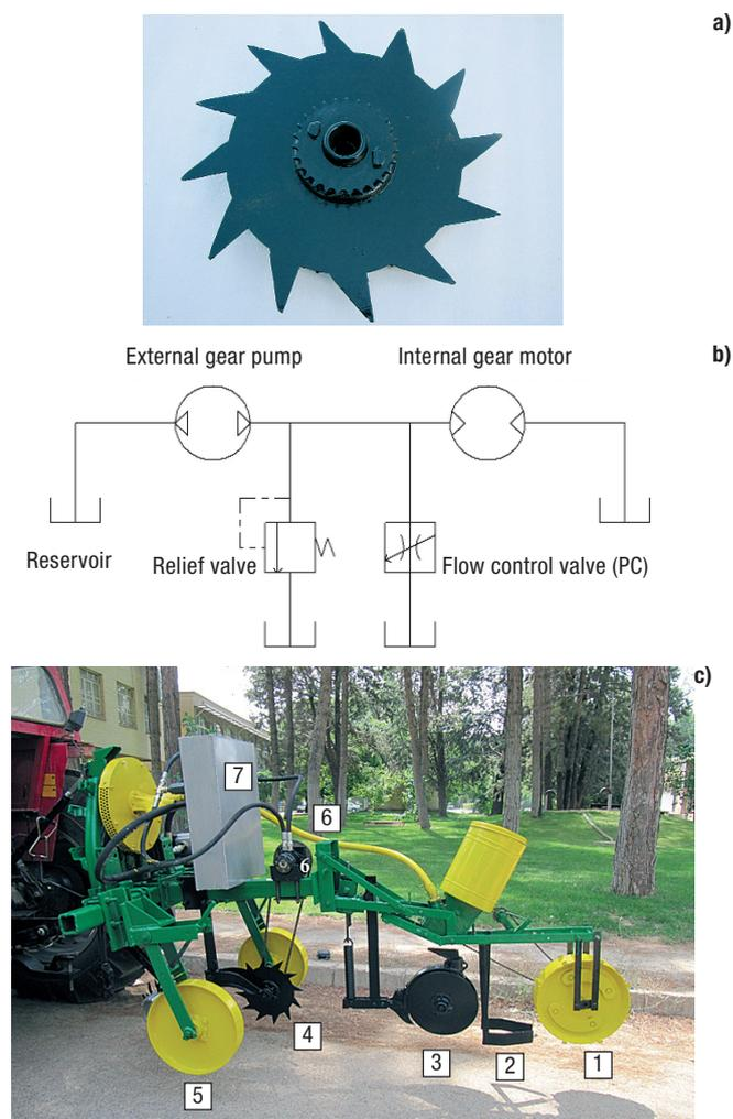
**Figure 1.** The fabricated toothed coulters (a), layout of the hydrostatic system (b) and row crop planters (c) used in this study: 1) drive wheel of the seed metering; 2) furrow filler; 3) double disk furrow opener; 4) toothed coulters; 5) gauge wheel; 6) hydro motor; 7) reservoir.
