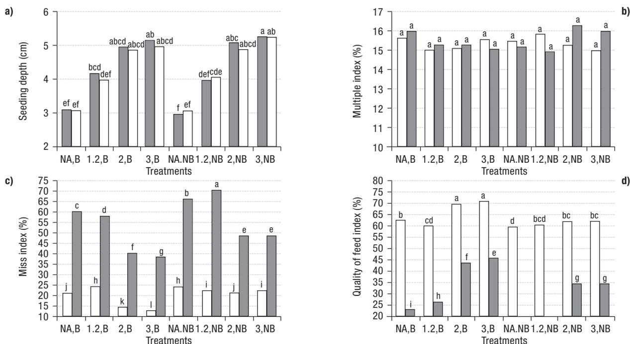
**Figure 2.** Comparison of means of (a) seeding depth, (b) multiple index (c) miss index, and (d) quality of feed index at various residue conditions, speed ratios and attachment modes. NB, non-baled residue; B, residue removed by baling; NA, inactive coultter (control); 1, 2 and 3, speed ratios; RC, with row cleaner; NRC, without row cleaner. Columns with same letters are not significantly different at  $p < 0.05$ . Grey histograms: RC. White histograms: NRC.
