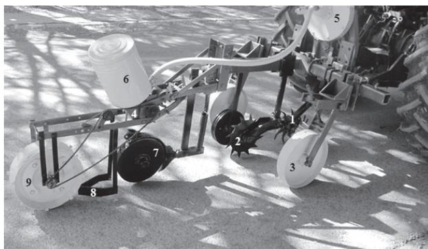
**Figure 2.** Mounted pneumatic row-crop planter used in this study: 1, row cleaner attachment; 2, toothed coulter; 3, gauge wheel; 4, pneumatic seed metering unit; 5, vacuum fan; 6, seed hopper; 7, double disk furrow opener; 8, furrow filler; 9, press-wheel drive.
