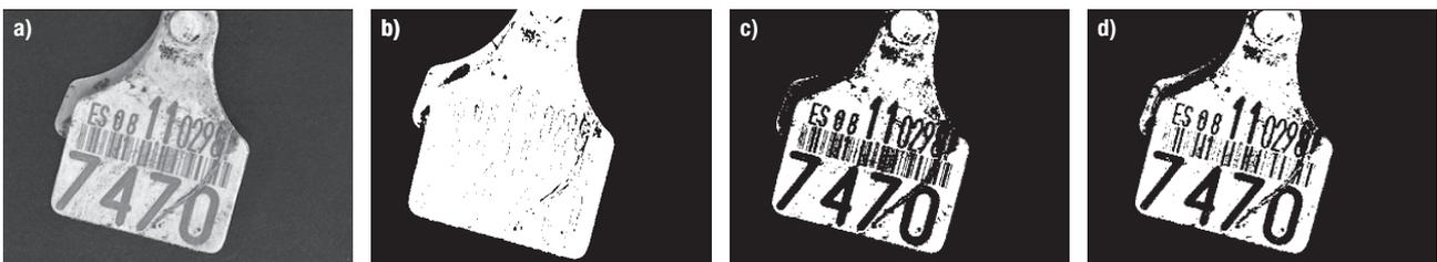
**Figure 6.** Sample captured ear-tag image: (a) original grey-level image, (b) Otsu binarization, (c) result after Log LRT thresholding and (d) result after  $k$ -means thresholding.
